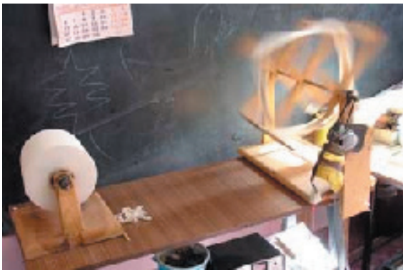
Skein winder with electric motor. This tool is only for winding skeins.
