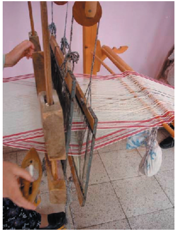
The mechanism of a simple treadle loom. The wooden rods seen on the right keep the warp in order. Foot pedals operate the wire heddles to separate the warp. On the left is the comb-like reed which presses the new weft thread firmly against the previous one.
